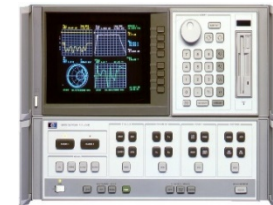
1984 | 8510A vector network analyzer
